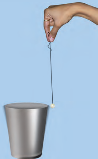
Fig. 13.17 : Thermocol ball touching the vibrating glass tumbler
