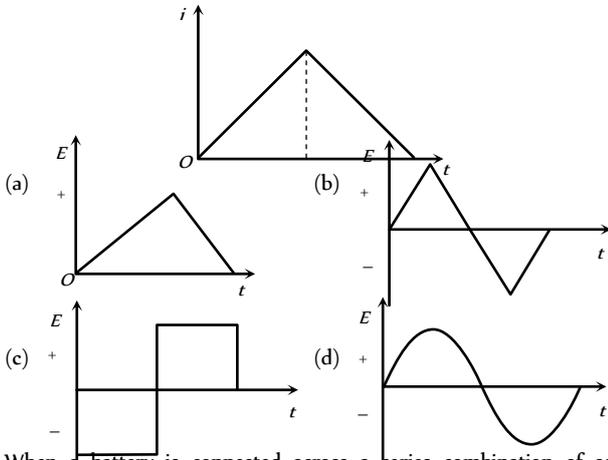
11. When a battery is connected across a series combination of self inductance  $L$  and resistance  $R$ , the variation in the current  $i$  with time  $t$  is best represented by [MP PET 2004]
