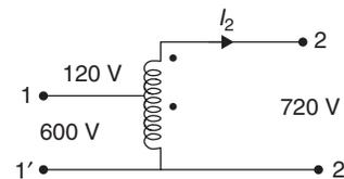
Maximum load can be supplied, if the two windings are connected in additive polarity as shown in above figure.
