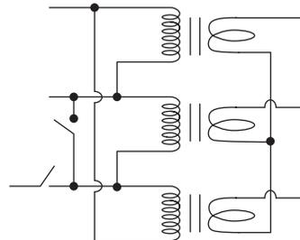
Transformer is used to step down voltage from 11000 V to 415 V line to line. Normally  $S_1$  is closed and  $S_2$  is open. If  $S_1$  is open and  $S_2$  is closed, what is the voltage across a and c?
