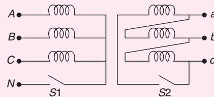
The star-delta transformer shown above is excited on the star side with a balanced, 4-wire, 3-phase, sinusoidal voltage supply of rated magnitude. The transformer is under no load condition.
