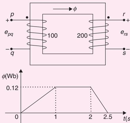
The induced emf ( $e_{rs}$ ) in the secondary winding as a function of time will be of the form
