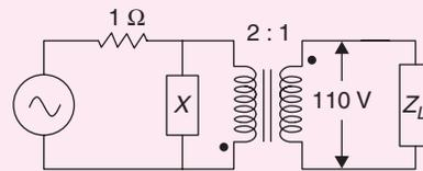
Assuming the transformer to be ideal, the value of the reactance  $X$  to improve the input power factor to unity is \_\_\_\_\_. [2014]
