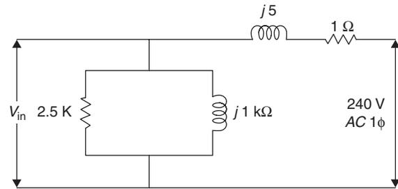
46. Equivalent circuit of 240/110 V 1.2 kVA single-phase transformer referred to primary. Delivers full load at rated voltage and u.p.f. Efficiency will be
