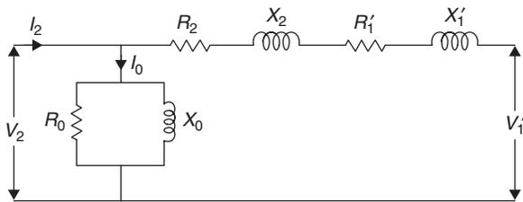
**Example 4:** A 15 kVA, 2300/230 V, 50 Hz single-phase transformer gave the following test data.
