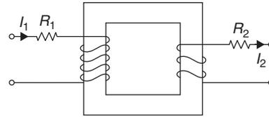
In the above figure, a transformer is shown whose primary and secondary windings have resistances of  $R_1$  and  $R_2$ , respectively.
