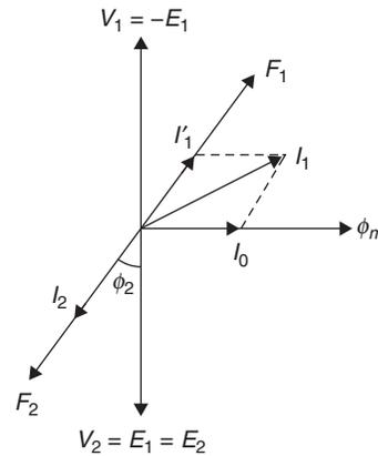
**Figure 1** Phasor diagram of ideal transformer for inductive load
