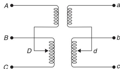
If the two transformers are of identical voltage ratings, one of the transformers has centre taps both on the primary and
