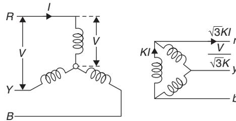
The main use of this connection is at the substation end of the transmission line where the voltage is to be stepped down. The primary winding is star connected with grounded neutral.
