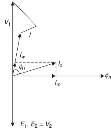
The no-load primary current  $I_0$  is called the exciting current of the transformer and can be resolved into two components.
