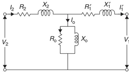
Approximate equivalent circuit referred to the secondary is shown in figure.
