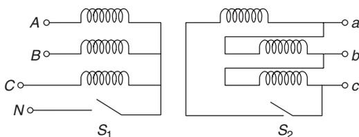
The star-delta transformer shown above is excited on the star side with balanced, 4-wire, 3-phase, sinusoidal voltage supply of rated magnitude. The transformer is under no load condition.
