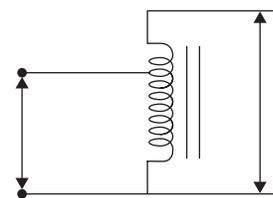
50 kVA 3300/230 V transformer is reconnected as an auto-transformer. The nominal rating of auto-transformer would be
