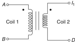
The figure above shows coils 1 and 2, with dot markings as shown, having 2000 and 3000 turns, respectively. Both the coils have a rated current of 25 A. Coil-1 is excited with single phase, 400 V, 50 Hz supply.
