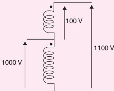
The kVA rating of the auto-transformer is \_\_\_\_\_. [2014]
