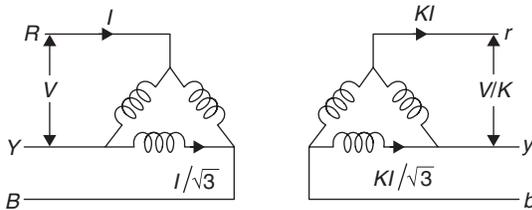
This connection is economical for large, low voltage transformers in which insulation problem is not so urgent, because it increases number of turns/phase.
