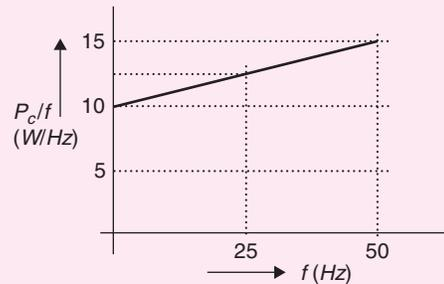
The hysteresis and eddy current losses of the transformer at 25 Hz, respectively, are [2014]
