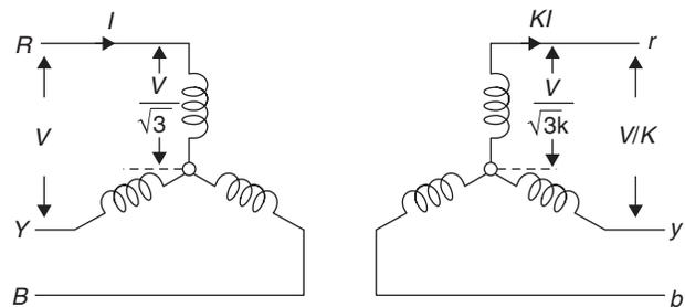
This connection is most economical for small, high-voltage transformers because the number of turns/phase and the amount of insulation required is minimum (as phase voltage is only  $1/\sqrt{3}$  of line voltage). The ratio of line voltages on the primary and secondary is the same as the transformation ratio of each transformer.
