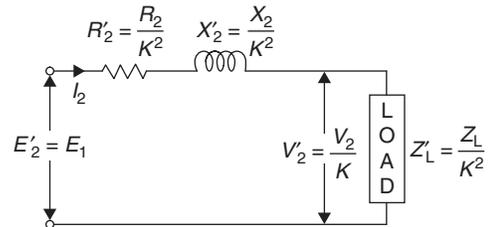
The total equivalent circuit of the transformer is obtained by adding in the primary impedance as shown in the following figure. This is known as exact equivalent circuit. A simplification can be made by transferring the existing circuit across the supply terminals as shown in below figure.
