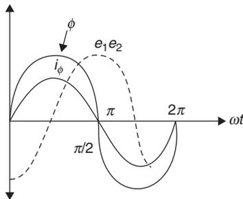
When secondary of transformer is loaded, the load will draw secondary current  $I_2$ , which sets up  $N_2 I_2$ , the secondary MMF and it opposes the main flux  $\phi_m$ . The secondary MMF  $F_2$  weakens the main flux  $\phi_m$ . But any reduction in  $\phi_m$  reduces  $E_1$  and in case of ideal transformer  $V_1 = -E_1$ . Hence, an extra load component of current  $I_1'$  is drawn by primary to compensate the secondary ampere-turns to maintain constant core flux.
