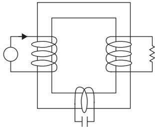
$N_1:N_2:N_3 = 4:2:1$ ,  $V_1 = 400 \angle 0$ . The current phasor in  $N_1$ ,  $I_1$  is given by
