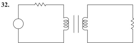
In the figure, transformer is ideal. For what number of turns in primary, maximum power is transferred.
