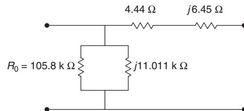
**Example 5:** A 3300/230 V, 50-kVA transformer is found to have impedance of 4% and a Cu. loss of 1.8% at full load. Find its percentage reactance and also the ohmic values of resistance, reactance and impedance as referred to primary. What would be the value of primary short-circuit current if primary voltage is assumed constant?
