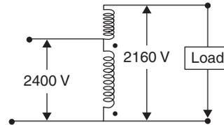
Here  $V_2 = 2400 - 240 = 2160 \text{ V}$
