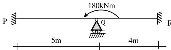
The rotation at Q (in rad, up to two decimal places) is \_\_\_\_\_
