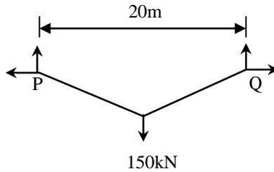
Neglecting the self weight of the cable. The tension (in kN. In integer value) in the cable due to the applied load will be \_\_\_\_\_.
