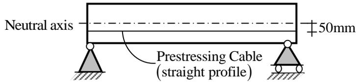
The beam carries a uniformly distributed load of 6kN/m over its entire span. If the effective flexural rigidity  $EI=2 \times 10^4 \text{ kNm}^2$  and the effective prestressing force is 200kN, the net increase in length of the prestressing cable (in mm, up to two decimal places) is \_\_\_\_\_.
