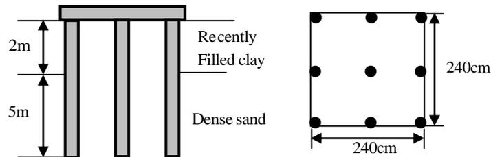
The negative frictional load (in kN, up to two decimal places) acting on the pile group is \_\_\_\_\_.
