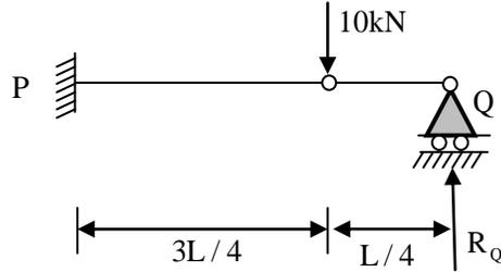
The vertical reaction at support Q is
