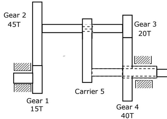
74. What is the relation between the angular velocities of Gear 1 and Gear 4?
