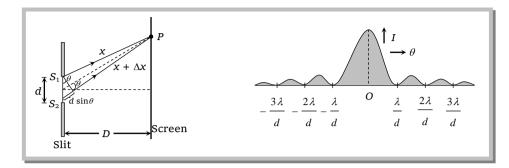
(i) Width of central maxima  $\beta_0 = \frac{2\lambda D}{d}$ ; and angular width  $= \frac{2\lambda}{d}$
