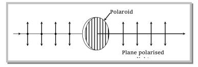
(i) Polaroids allow the light oscillations parallel to the transmission axis pass through them.
