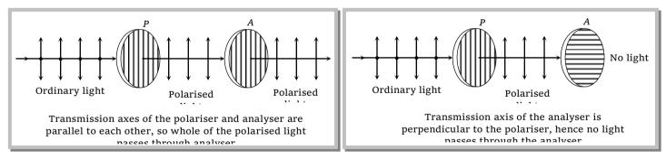
**Note** : UP When unpolarised light is incident on the polariser, the intensity of the transmitted polarised light is half the intensity of unpolarised light.
