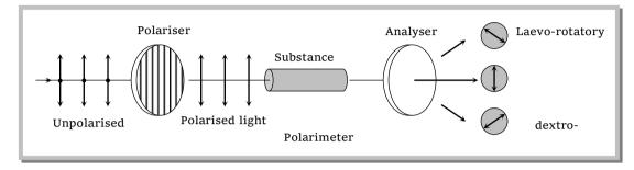
The optical activity of a substance is related to the asymmetry of the molecule or crystal as a whole, *e.g.*, a solution of cane-sugar is dextro-rotatory due to asymmetrical molecular structure while crystals of quartz are dextro or laevo-rotatory due to structural asymmetry which vanishes when quartz is fused.
