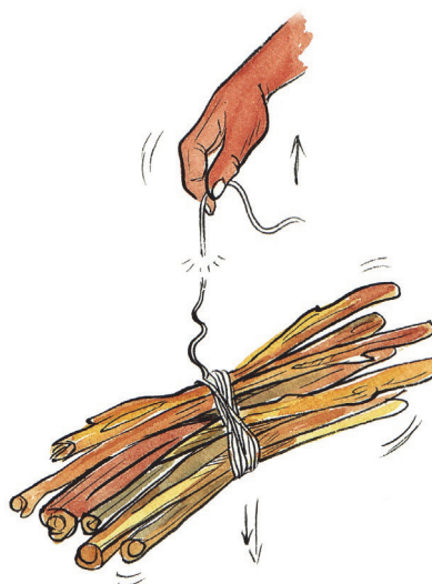
Fig. 10.8 The string breaks when the bundle is lifted quickly.
