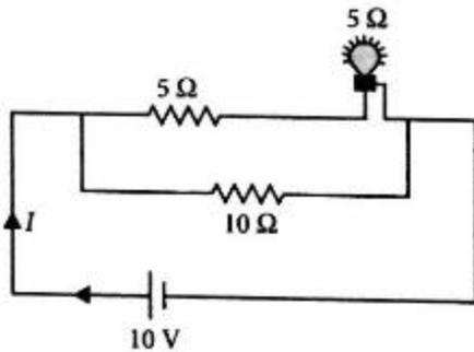
$$\text{Net resistance of the circuit} = \frac{10 \times 10}{10 + 10} = 5 \Omega$$
