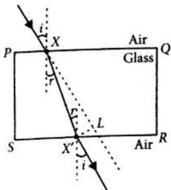
As can be seen that at points X and X', the incident ray, the refracted ray and the normal all lie in the same plane.
