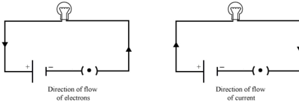
Conventionally, the direction of an electric current is taken as opposite to the direction of an electric charge. Hence, electric current flows from the positive terminal to the negative terminal via the bulb.
