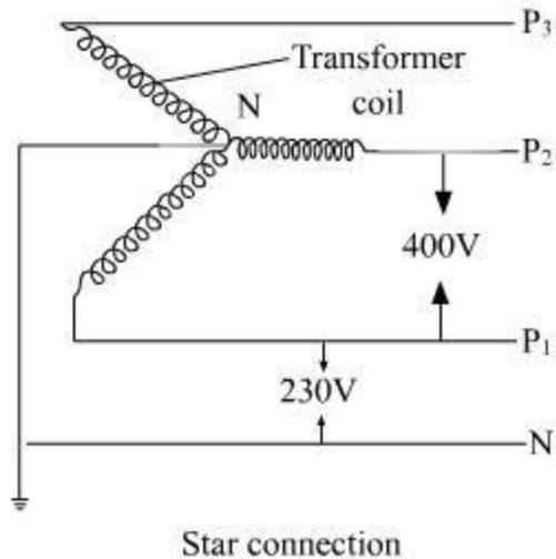
We get four lines out of the distribution transformer; three phase lines ( $P_1, P_2$  and  $P_3$ ) and one neutral line ( $N$ ). Each phase has the same frequency but different voltages.
