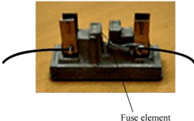
To prevent any damage by short circuiting or over loading, an electric fuse (that consists of a low melting point wire) is used. The wiring of the circuit is made of low resistance copper wire of a certain thickness. This allows only a maximum amount of current to flow through it, which is called its **safe limit**.
