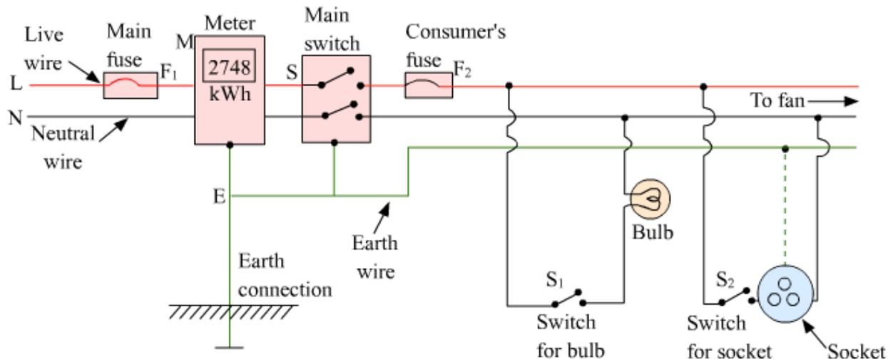
In the above diagram, the pair of wires L and N first enter the main box, which is placed outside the house. From here, live wire L goes into the main fuse  $F_1$  having a high rating of about 50 A.
