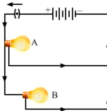
**In domestic circuit, parallel circuit is always preferred over series circuit.**
