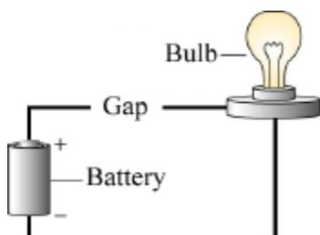
Construct a simple electrical circuit, as shown in the given figure.
