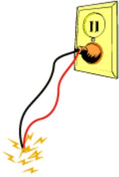
Short circuiting occurs when naked live and neutral wires touch each other. In such a case, the resistance of the circuit becomes very less. Now, according to Ohm's law, current is inversely proportional to resistance.
