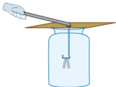
Touch a charged glass rod with the metal strip of an electroscope. You will observe that the aluminum strips are repelled by each other. Also, you will observe that they remain in that position even after removing the glass rod. Now, touch the metal strip with your hand. **What do you observe?**
