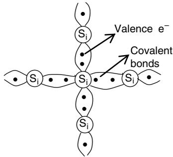
Figure 3 crystalline structure of Si
