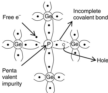
Figure 4 Crystalline structure of N-type semiconductor
