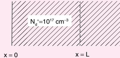
Given  $q = 1.6 \times 10^{-19}$  coulomb,  $\epsilon_0 = 8.85 \times 10^{-14}$  F/cm,  $\epsilon_r = 11.7$  for silicon, the value of  $L$  in nm is \_\_\_\_\_ .
