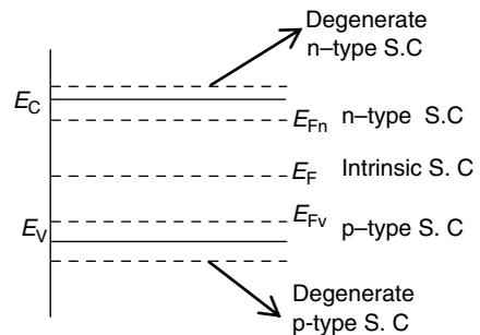
If temperature  $T$  increases, the Fermi levels of p-type and n-type semiconductor moves towards the middle of the forbidden energy band.
