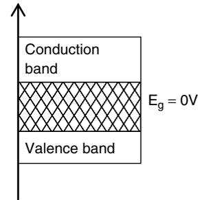
Figure 2 Energy band diagrams
