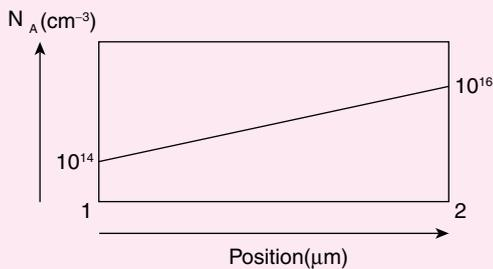
The magnitude of the electric field (in kV/cm) in the semiconductor due to non uniform doping is \_\_\_\_\_ . [2016]
