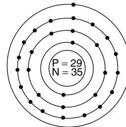
Figure 1 Structure of copper atom
