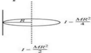
Moment of inertia of disc about passing through a point of its edge is given by;
