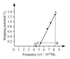
It can be observed that the obtained curve is a straight line. It intersects the *v*-axis at  $5 \times 10^{14}$  Hz, which is the threshold frequency ( $v_0$ ) of the material. Point D corresponds to a frequency less than the threshold frequency. Hence, there is no photoelectric emission for the  $\lambda_5$  line, and therefore, no stopping voltage is required to stop the current.
