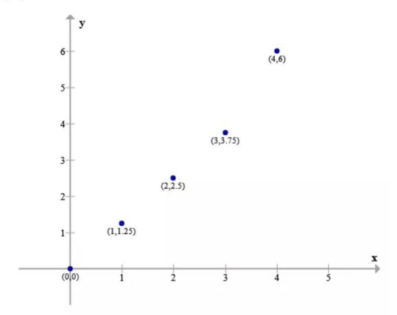
The graph consists of separate points, so the function is discrete.
