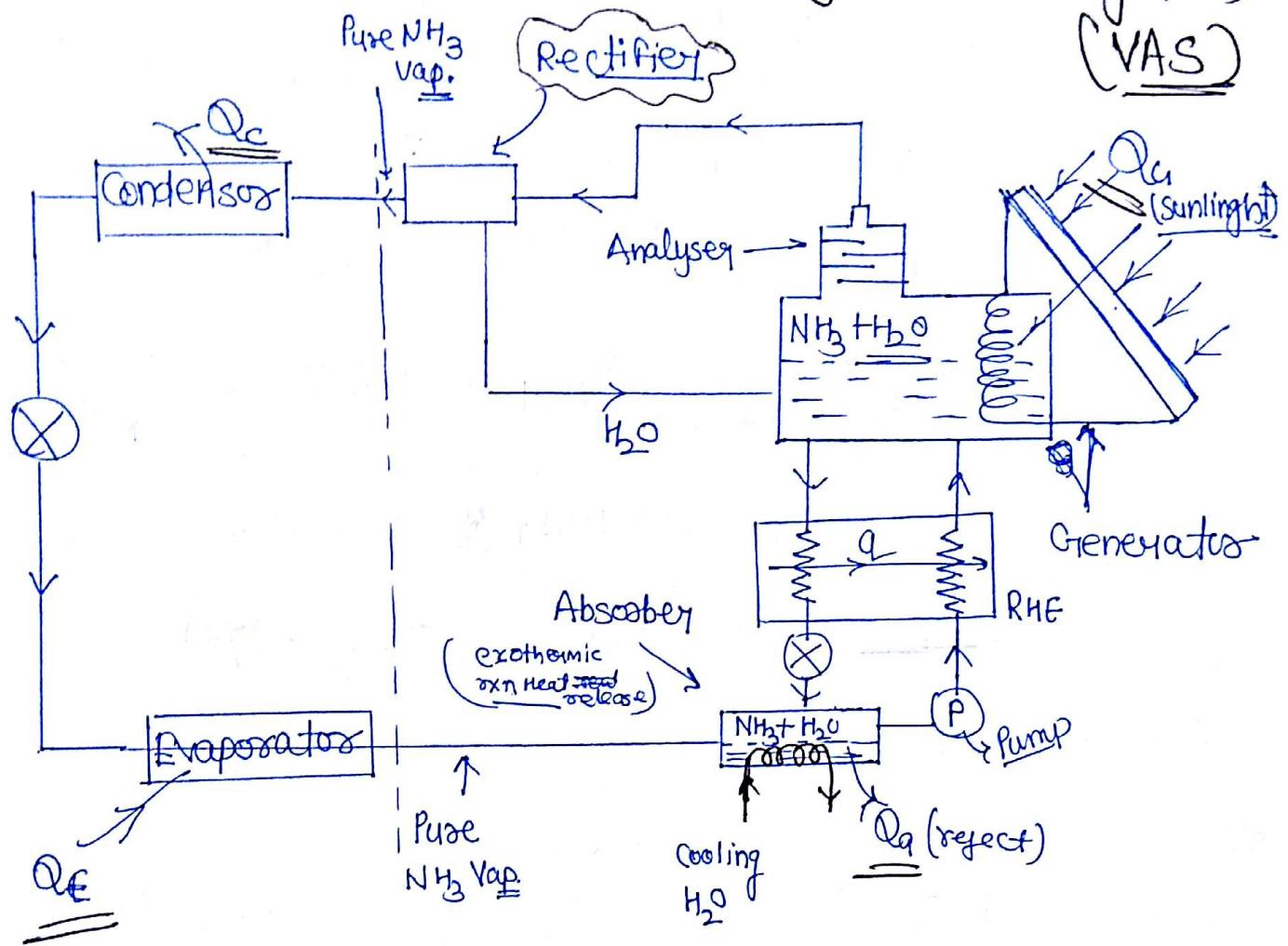
→ Pure NH<sub>3</sub> vapour enters the absorber where it is absorbed in water (H<sub>2</sub>O). The reaction is exothermic and the solubility of NH<sub>3</sub> is inversely proportional to temp. of solution. Cooling water is continuously circulating to maintain a low temp. of solution to facilitate absorption of NH<sub>3</sub>. Solution rich in NH<sub>3</sub> is pumped to Generator via Regenerative heat exchanger in Generator this solution absorbs heat and NH<sub>3</sub> separates
