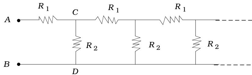
In the following figure, a circuit of an infinitely long series network of resistors is shown. Find the equivalent resistance of network between the points A and B, when  $R_1 = 1 \Omega$  and  $R_2 = 2 \Omega$  : 2
