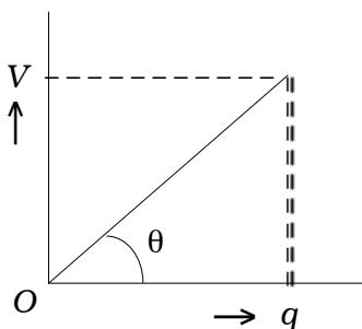
A graph between potential ( $V$ ) and charge ( $q$ ) of an isolated sphere is shown in figure. Capacitance of the sphere will be
