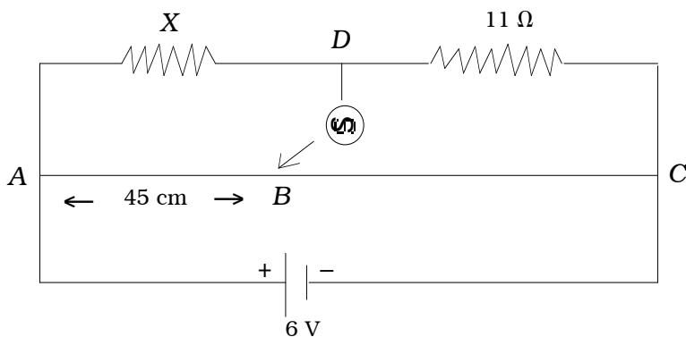
In figure, a meter-bridge is shown in its balance position. Find the value of unknown resistance ( X ).
