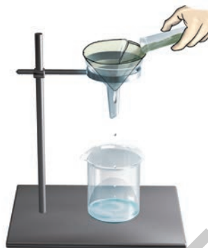
Fig. 5.10 Filtration using a filter paper
