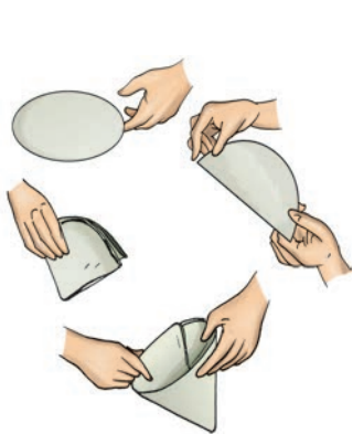
Fig. 5.9 Folding a filter paper to make a cone
