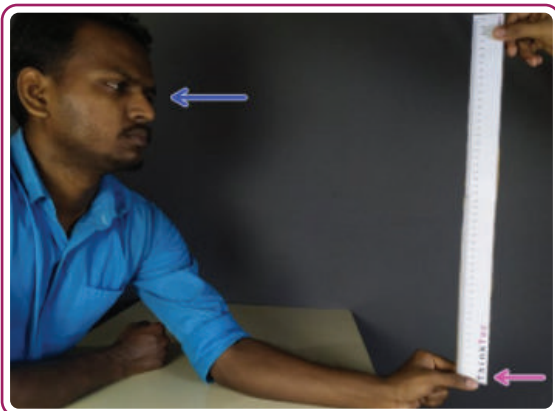
Fig. 3.2 , Shyam was asked to rest his hand on a surface and stretch his thumb and forefinger parallel to the zeroth mark of a 1 m ruler, held vertically by Rizwan.
