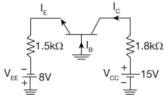
For the common base circuit shown in figure, then find the value of  $V_{CB}$ .
