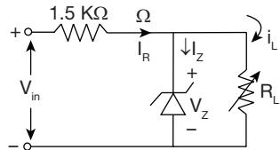
Consider  $V_{in} = 40\text{ V}$ ,  $V_z = 10\text{ V}$  and  $I_{zM} = 15\text{ mA}$
