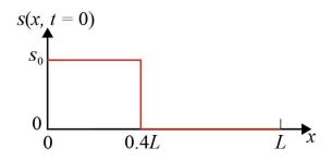
The boundary conditions of the problem are given by  $\frac{\partial s(x,t)}{\partial x} = 0$  at the boundary points  $x = \mathbf{0}$  and x = L at all times. Consider  $D = \mathbf{0.1 m^2/s}$ ,  $s_0 = \mathbf{5 \mu mol/m}$ , and  $L = \mathbf{10 m}$ .
