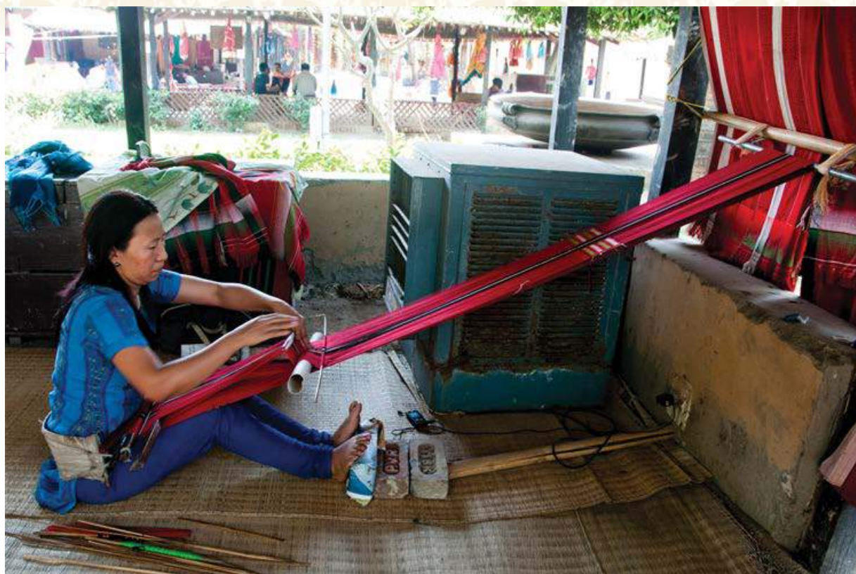
Pic. 5.11: Back strap loom
