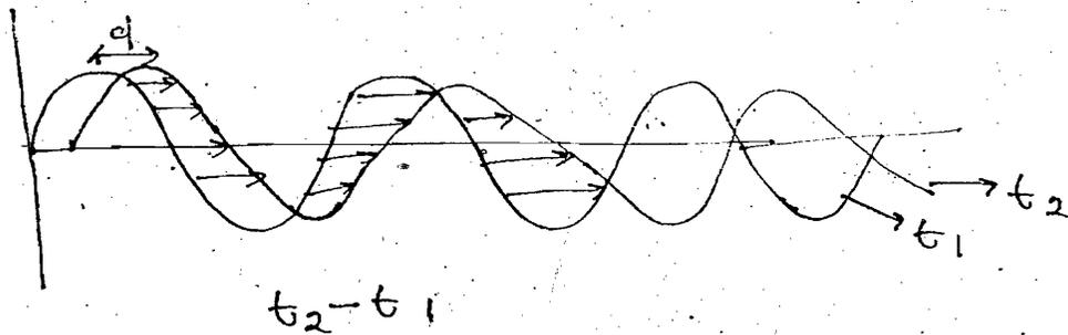
The distance travelled by any in-phase point per unit time is called as phase velocity.
