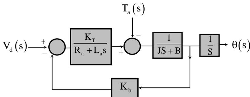
The values of the parameters are  $K_T = 1 \text{ N-m/A}$ ,  $R_a = 1 \Omega$ ,  $L_a = 0.1 \text{ H}$ ,  $J = 5 \text{ kg-m}^2$ ,  $B = 1 \text{ N-m (rad/sec)}$  and  $K_b = 1 \text{ V/(rad/sec)}$ . The steady-state position response (in radians) due to unit impulse disturbance torque  $T_{dis}$  \_\_\_\_\_.
