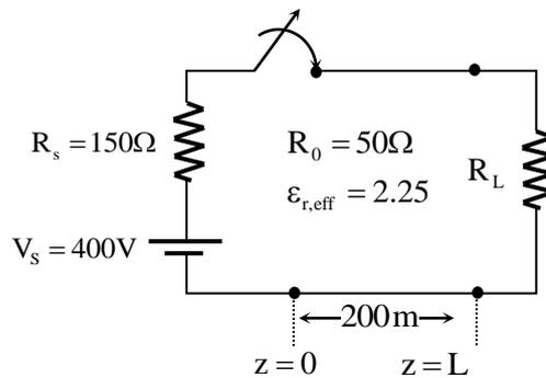
The transient response of the circuit at the input of the line ( $z = 0$ ) is also drawn in the figure. The value of  $R_L$  (in  $\Omega$ ) is \_\_\_\_\_.
