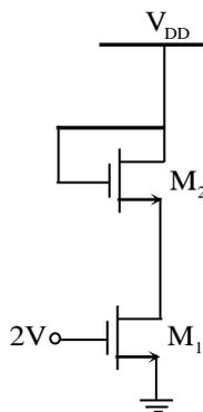
Assume that the channel length modulation parameter  $\lambda$  is zero and body is shorted to source. The minimum supply voltage  $V_{DD}$ (in volts) needed to ensure that transistor  $M_1$  operates in saturation mode of operation is \_\_\_\_\_.
