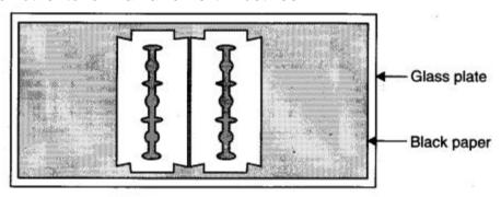
A thin slit made by using two razor blades, black paper and a glass plate.
