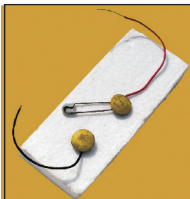
Fig 12.8 A simple switch with a switch
