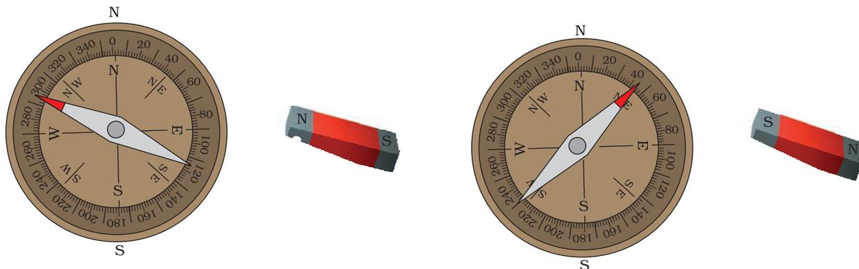
17. **Hint:** Magnetise the needle and set it in a way that it may rotate freely suspend it.
