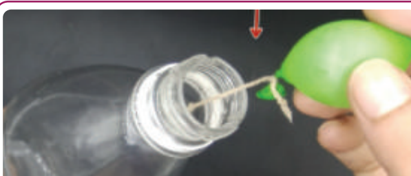
Fig. 5.5, Carefully insert the balloon and magnet into a plastic bottle through its mouth.
