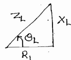
$$P_L = \frac{V_{th}^2 Z_L \cos \theta_L}{(Z_L \cos \theta_L + R_{th})^2 + (Z_L \sin \theta_L + X_{th})^2} \quad (III)$$
