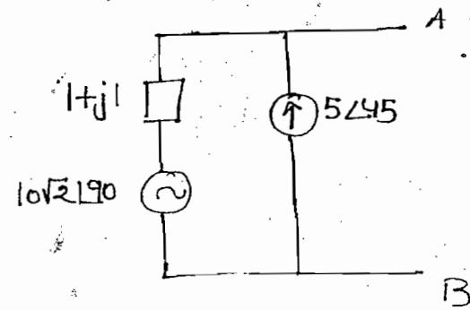
$$I_1 = \frac{10\sqrt{2} \angle 190^\circ}{\sqrt{2} \angle 45^\circ} = 10 \angle 45^\circ$$
