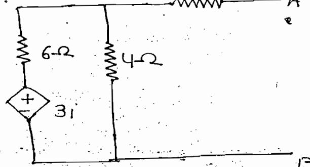
$$i = \frac{V_1 - 1}{1} \Rightarrow V_1 = \frac{6}{11}$$
