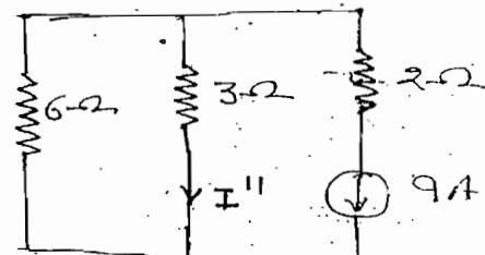
Ques:- Find  $V_x$  by using superposition theorem
