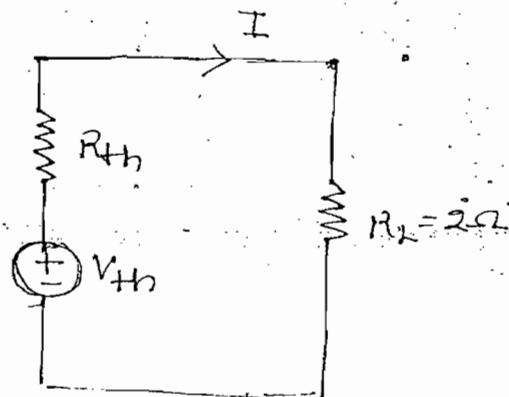
ques:- When a battery charger connected to  $1\Omega$  resistor, current in the resistor is 5A. When same battery charger is connected for charging of ideal 2V battery at 7A rate. Find  $V_{th}$  &  $R_{th}$
