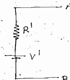
$$V_{Th} = I_{Sc} R_{Th}$$
