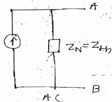
Ques:- Find current in  $1\Omega$  resistor using Norton's theorem
