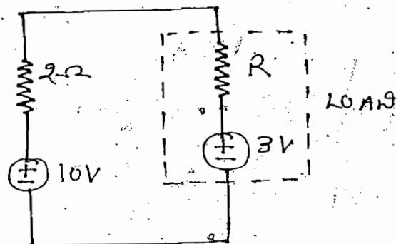
$$\text{soln}:- (R_{\text{req}})_L = R_S = 2\Omega$$
