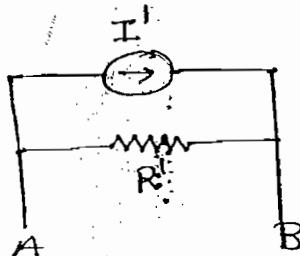
$$I_{sc} = \frac{V_{oc}}{R_{th}}$$
