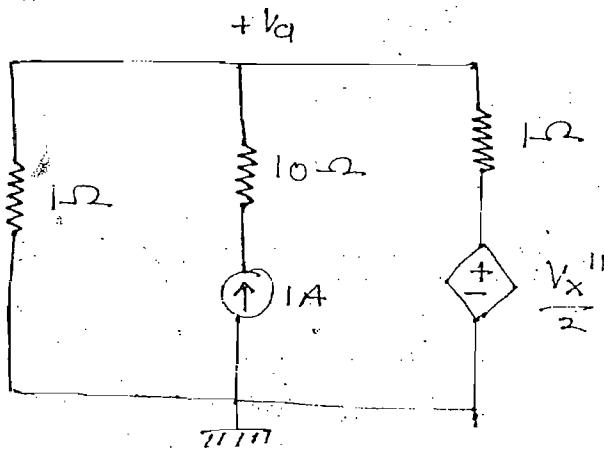
Ques:- In the circuit shown power dissipation in 1Ω resistor is 576W when voltage source is acting along and power dissipation in 1Ω is resistor is 1W when current source is acting along. Find total power dissipation in 1 ohm resistor
