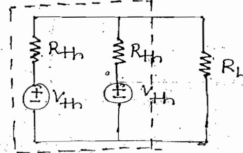
$$I' = \frac{V_{th}}{R_L + \frac{R_{th}}{2}} = \frac{2V_{th}}{2R_L + R_{th}}$$
