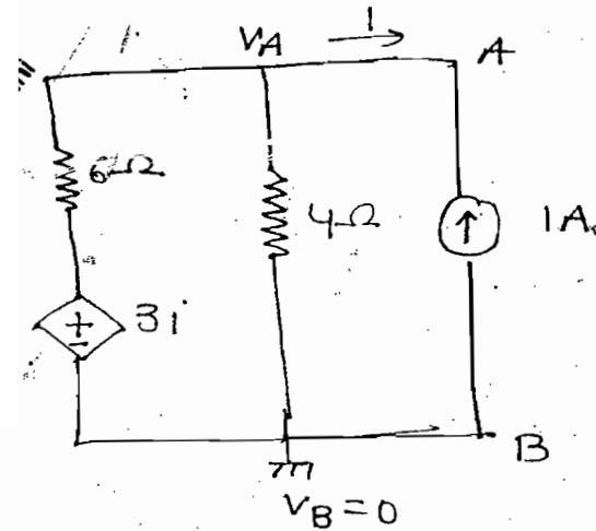
$$R_{th} = \frac{V_{AB}}{I_s} = \frac{1.2}{1} = 1.2 \Omega, \text{ Ans}$$
