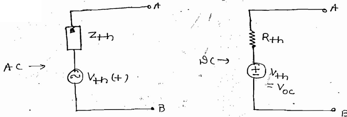
When N/w is having linear bidirectional elements and more no. of active and passive elements, it can be replaced by single equivalent circuit consisting of equivalent voltage source ( $V_{th}$ ) in series with equivalent resistance ( $R_{th}$ )
