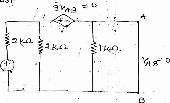
$$R_{TH} = \frac{V_{OC}}{I_{SC}} = \frac{0.5}{\frac{5}{2 \times 10^3}} = 200\Omega$$
