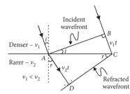
Let the angles of incidence and refraction be i and r respectively.
