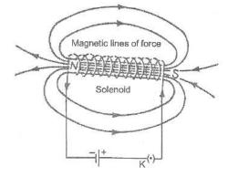
The magnetic field, thus produced, is very much similar to that of a bar magnet and one end of the coil acts like a magnetic north pole, while the other acts like a south pole.
