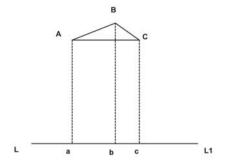
Figure 6.12 Orthogonal projection
