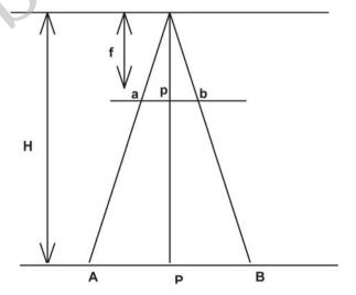
Figure 6.15 Focal Length of the Camera (f) and Flying Height of the Aircraft (H)
