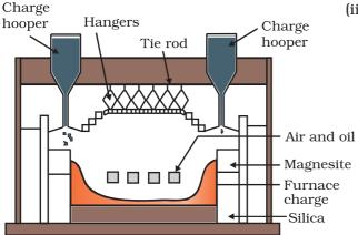
Fig. 6.3: A section of a modern reverberatory furnace
