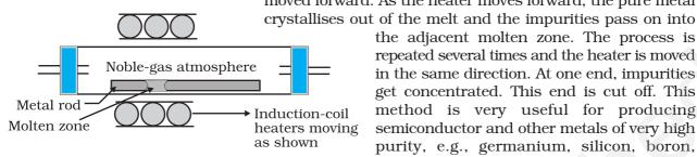
Fig. 6.7: Zone refining process
