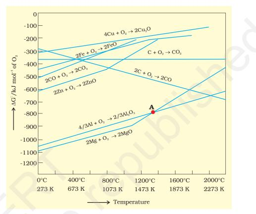
**Fig. 6.4:** Gibbs energy  $(\Delta G^{\circ})$  vs T plots (schematic) for formation of some oxides (Ellingham diagram)
