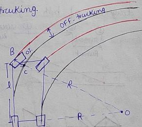
Mechanical widening is provided to account off-tracking
