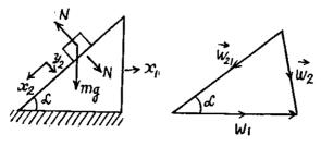
1.82 To analyse the kinematic relations between the bodies, sketch the force diagram of each body as shown in the figure.
