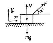
$$m\int_{0}^{r} dv_{x} = a \cos \alpha \int_{0}^{r} t dt \quad \text{(using Eq. 1)}$$
