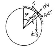
1.108 In the problem, we require the velocity of the body, realtive to the sphere, which itself moves with an acceleration  $w_0$  in horizontal direction (say towards left). Hence it is advisible to solve the problem in the frame of sphere (non-inertial frame).
