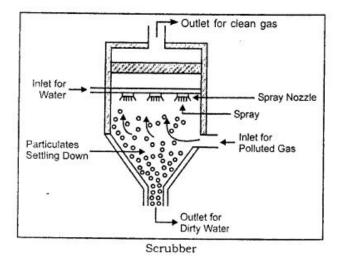
during emissions. In this process, water is introduced into a spray tower by means of a spray nozzle which allow downward flow of water. As the polluted gas flows upwards, the particulates present in the gas collide with the water droplets being sprayed from the spray nozzles. Under the influence of gravitational force, the liquid droplets containing the particulates settle at the bottom.
