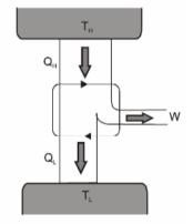
Efficiency ,  $\eta = \frac{\text{work done by the engine}}{\text{heat sup plied to it}}$
