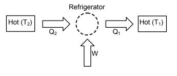
• Coefficient of performance,  $\beta = \frac{Q_2}{W} = -\frac{1}{\frac{T_1}{T_2} - 1} = -\frac{1}{\frac{T_1}{T_2} - 1}$
