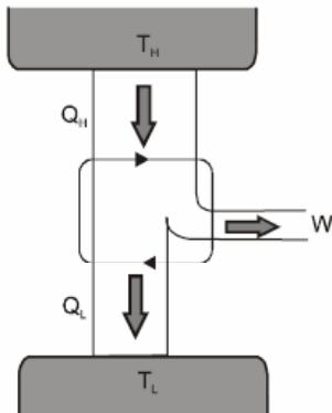
$$\text{Efficiency}, \eta = \frac{\text{work done by the engine}}{\text{heat supplied to it}}$$
