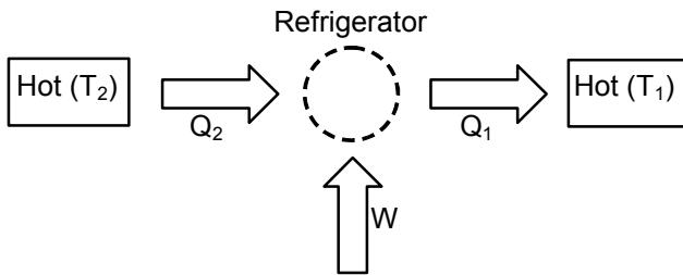
$$\bullet \text{ Coefficient of performance, } \beta = \frac{Q_2}{W} = \frac{1}{\frac{T_1}{T_2} - 1} = \frac{1}{\frac{T_1}{T_2} - 1}$$
