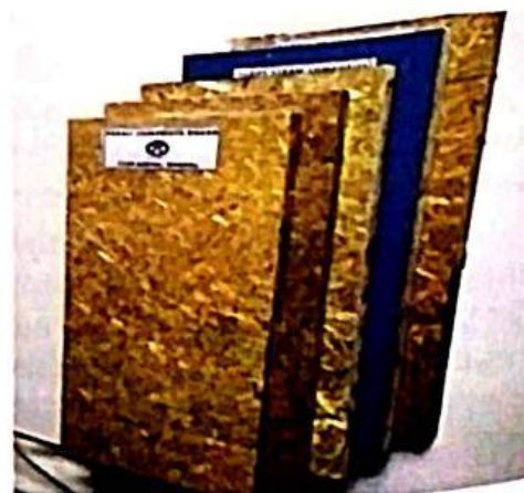
Technology Transfers to Industry - Converting parali (paddy stubble) straw into hybrid particleboard by CSIR.
