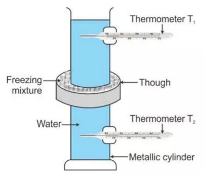
Hope's apparatus consists of a tall metallic cylinder provided with two side openings P and Q, P near the top and Q near the bottom, fitted with thermometers  $T_1$  and  $T_2$  in them. The central part of the cylinder is surrounded with a cylindrical trough containing a freezing mixture of ice and salt. The cylinder is fitted with pure water at room temperature.
