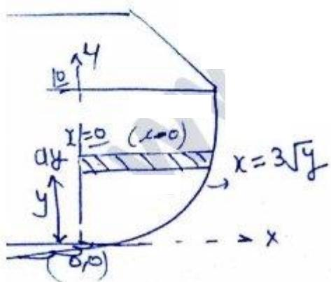
$$\begin{aligned} F_v &= \text{wt.} \\ &= \rho \times \text{Vol} \\ &= \rho \times A \times 1 \\ &= 9810 \times 2(10)^{3/2} \end{aligned}$$
