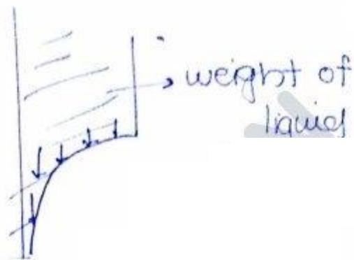
$F_v = \text{weight of liquid above wave surface.}$
