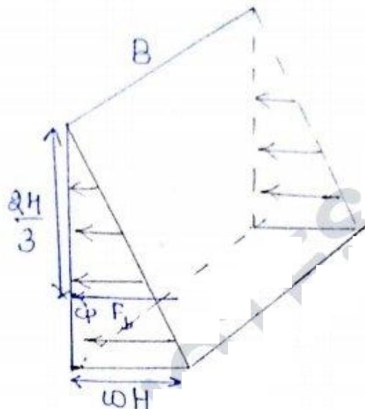
$$\begin{aligned} \text{Vol. of PD} &= \frac{1}{2} [\omega H \times H] \times B \\ &= \omega (H \times B) \times \frac{H}{2} \\ &= \omega \cdot A \cdot \bar{x} \end{aligned}$$
