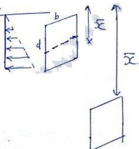
\* On vertical plane surface the pressure diagram become uniform as depth of immerse increase i.e. C.P. shifted towards C.G. of body but it will never coincide.
