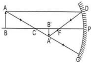
Object beyond C, a real, inverted diminished image between F and C, inverted at C and is of same size as that of object.
