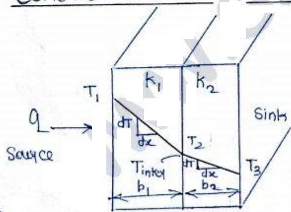
Assume! - steady state, one dimensional conduction H.T. through complete slab
