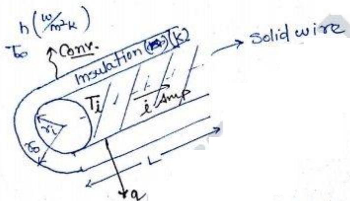
Consider a solid wire of Radius  $r_i$  inside which heat is being generated by passing electric power let an insulation having a thermal conductivity ( $k$ ) is being wrapped along wire upto the radius  $r_o$ . The Heat Generated in the wire is Radially Conducted through the insulation and than from the surface of insulation Heat is Convected to the Ambiant Air  $T_\infty$  with a Convective heat transfer coefficient  $h \text{ watt/m}^2\text{K}$
