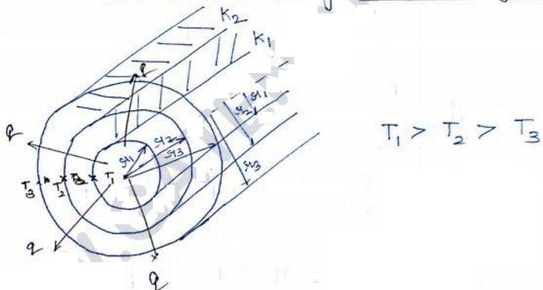
\* Since temp. Gradient are existing along radial direction Heat must be Conducting from the inner most Cylindrical Surface at  $T_1$  to outer most cylindrical surface at  $T_3$
