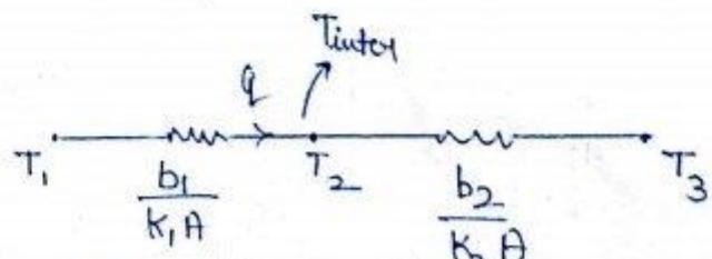
$\rightarrow k_1 < k_2$  because  $(\frac{dT}{dx})_{\text{inner}} \neq (\frac{dT}{dx})_{\text{outer}}$  ( $q$ ,  $A$  being same throughout)
