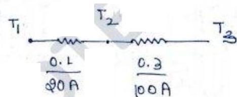
$$\frac{T_2 - T_3}{0.3 / 100\text{A}} = \frac{T_1 - T_2}{0.1 / 20\text{A}}$$
