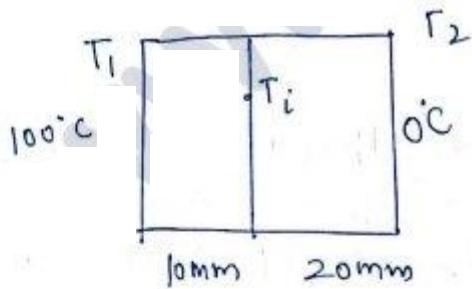
$$\frac{T_i - T_1}{\frac{10}{K_{Al}}} = \frac{T_i - T_2}{\frac{20}{K_{iron}}}$$
