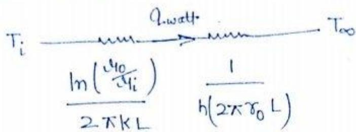
∴ Rate of Radial H.T. between wire and ambient
