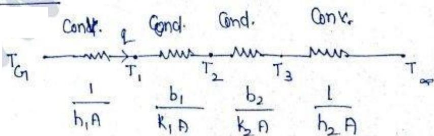
∴ Rate of Heat transfer between Hot Gases and ambient fluid
