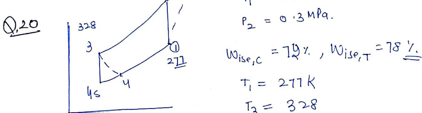
$$\frac{T_3}{T_{4S}} = \frac{T_{2S}}{T_1} \text{ or } T_{4S} = \frac{T_1}{\frac{T_{2S}}{T_1}}$$
