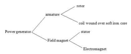
A power generator consists of two parts:
